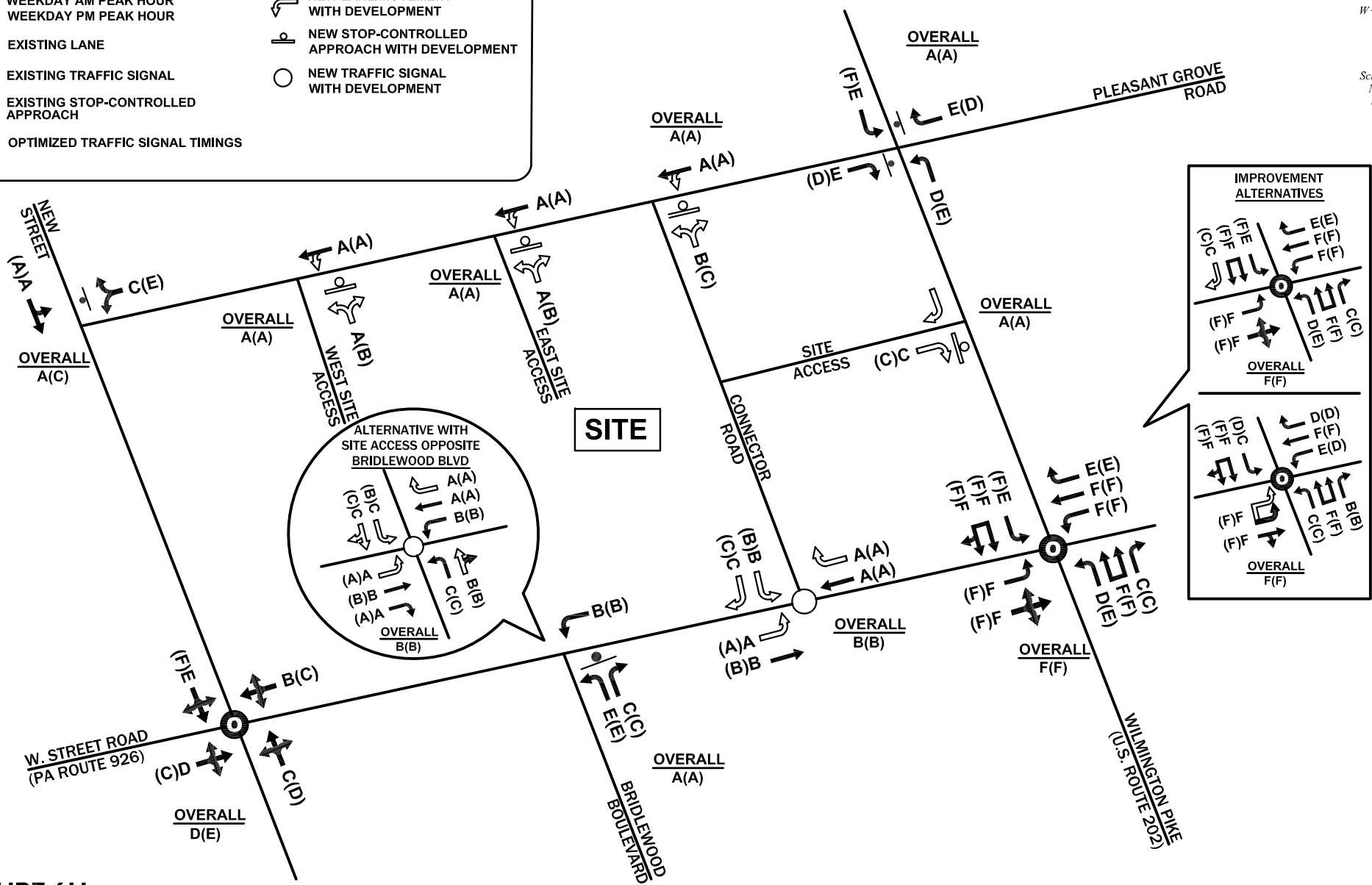
FIGURE 6H 2028 Future Peak Hour Levels of Service with Development Alternative C - 395 New Units with Provision of Connector Road
